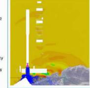
Approximately 200 million grid cells were used to capture the fine detail and geometry of the pad, and millions of particles were tracked to capture the dynamics of a water cascade. This work was performed using a density-based, finite-volume CFD code called Loci/CHEM.
